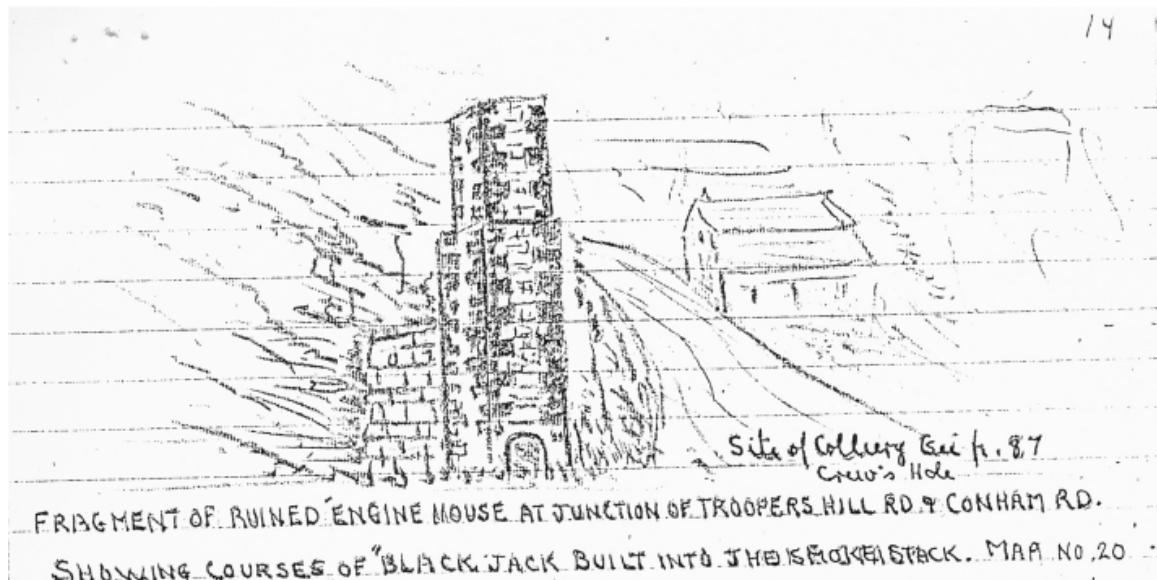
Site of Colliery Crew's Hole FRAGMENT OF RUINED 'ENGINE HOUSE' AT JUNCTION OF TROOPERS HILL RD & CONHAM RD. SHOWING COURSES OF "BLACK JACK" BUILT INTO THE SMOKE STACK. MAP NO. 20
